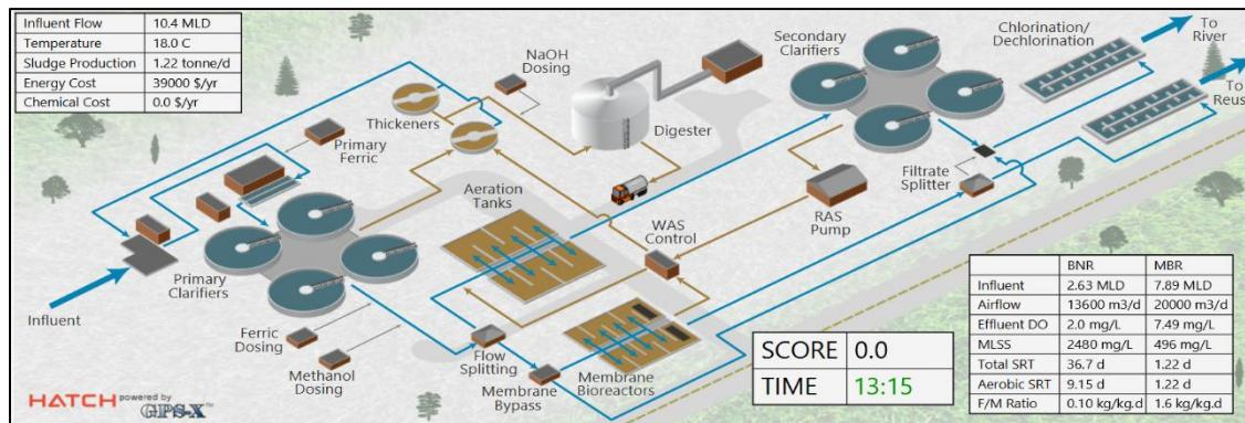
Note that there are two effluent points for this plant – one that goes to the river, and one that goes to water reuse. The activated sludge train can only discharge to the river, while the MBR train can discharge to either the river or the water reuse side. Note that there can be effluent targets for both effluent points for each challenge.
